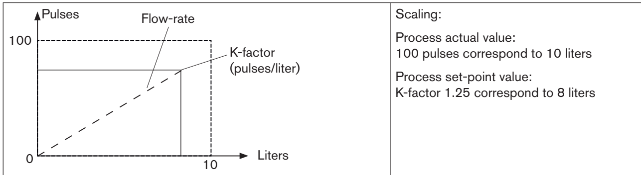
Figure 48: Example of a sensor calibration for frequency ( Frequenz ) signal type
