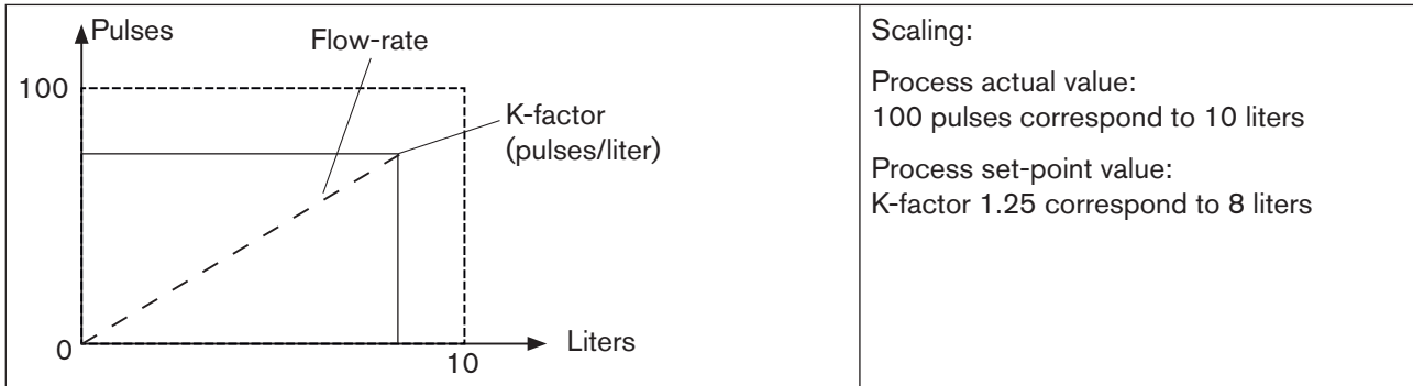
Figure 39: Example of a sensor calibration for frequency signal type
